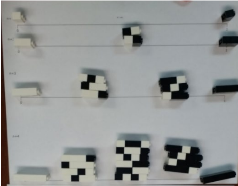
Figure 4.39. Theoretical permutations plots for 0-1 situation created by S using building blocks for sample sizes 1 (top) through 4 (bottom). Black represents a value of one and white represents a value of 0; each set of building blocks stuck together represents a possible sample whose mean is placed on the x-axis at its appropriate mean.
