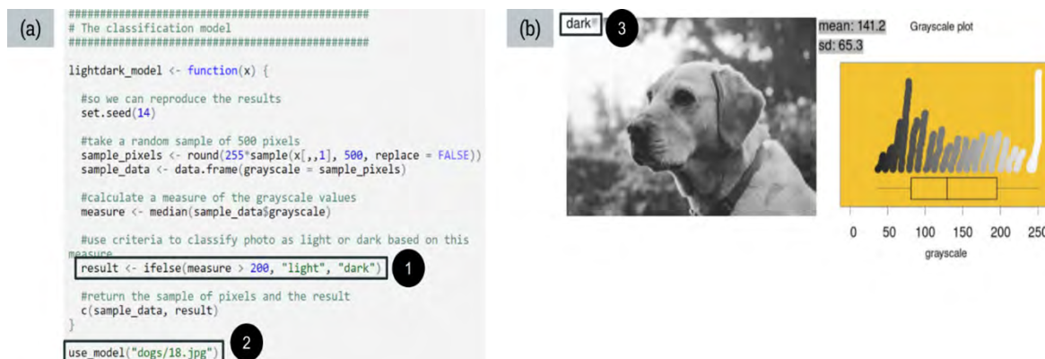
Figure 6.7: Example of a classification model articulated with code with the output generated from the model
